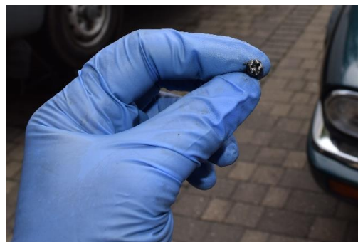
Figure 6 Screw with slot cut into the head
