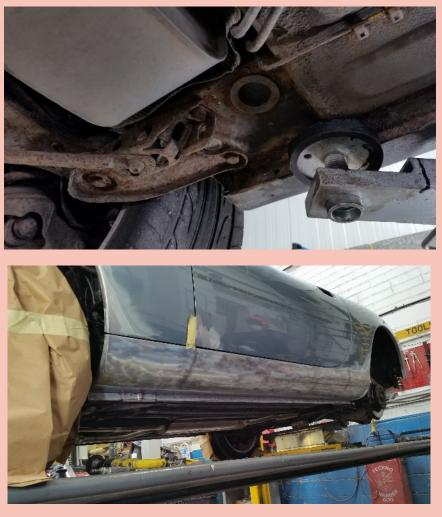
trapped between the inner wheel arch lip and the rear outer quarter panel which are bonded together with a foam like bonding. Most of the work will need a major removal of subframes and suspension at the front and rear of the car in order to get to the areas to take the necessary action to prevent serious corrosions of the chassis structure.
