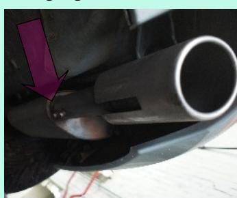
back from the box itself. Once both boxes were removed, the process of removing the tail pipes began. These are slotted onto the pipe exiting the silencer box. There are two allen key bolts securing the tailpipe to the exhaust tube on each
