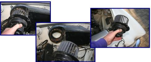
13) Take off the air filter to gain proper access under the bonnet and unscrew the five small bolts holding everything in and withdraw the fan/motor assembly.
