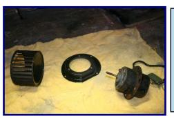
4) If you want to minimise the work under the bonnet, then it is best to assemble the new items on a workbench. You will therefore need the mounting plate from the practice heater. If not, then you will need to undertake items 1 to 3 on your heater on the car, but don't worry, it is accessible.
