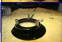
8) The fixing screws would then need to be replaced with correspondingly longer items.
