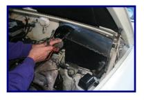
14) Offer up the new assembly and screw it in. A good tip here is to ensure that you shorten the new motor fixing lugs whilst still on the bench since they obstruct access to the fixing bolts. Presumably, the lugs are made longer so that they may fit other cars.
