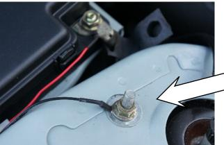
Then connect the black negative lead to one of the securing bolts for the suspension leg in order to get a
