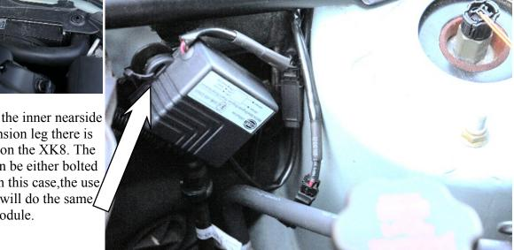
nearside wing. On the inner nearside wing by the suspension leg there is an unused bracket on the XK8. The sensing module can be either bolted to this bracket or in this case,the use of an electrical tie will do the same job securing the module.
