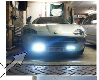
Once connected up, the Hella Daylight Running Lights should now work.
