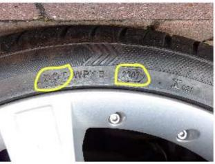
represent the week of the year it was made and the final two number indicate the last two digits of the year. See example: So the first two digits indicate that the tyre was made in the **26** Week and the last two indicate it was made in 2007. Prior to year 2000 there is three digits - first two are the week, the last one is the year: i.e. **128** indicates **12**th week of 1998. Isn't it about time you checked yours? **Doug Warren**
